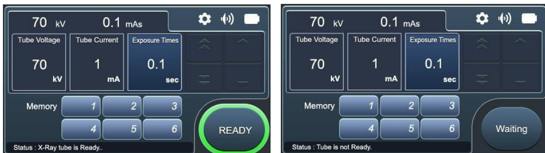
[Figure 7.9 Messages That Are Displayed When Generating an X-ray]
