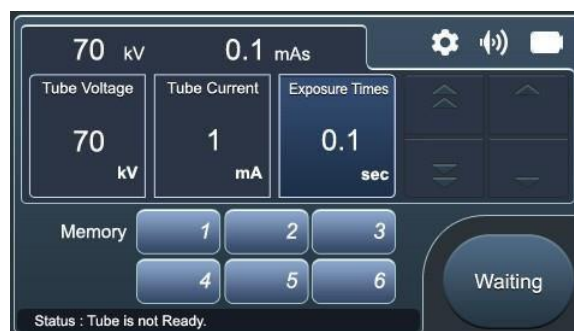
[Figure 7.12 Main Menu Screen After Radiation Is Emitted]
