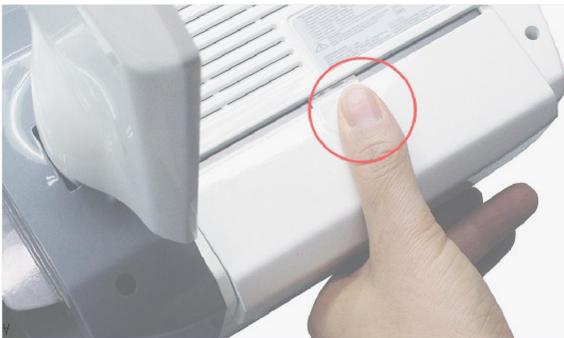
[Figure 7.15 Detaching the Battery Cover]
