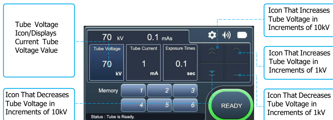
[ Figure 7.3 Icons to Change Tube Voltage Settings]
