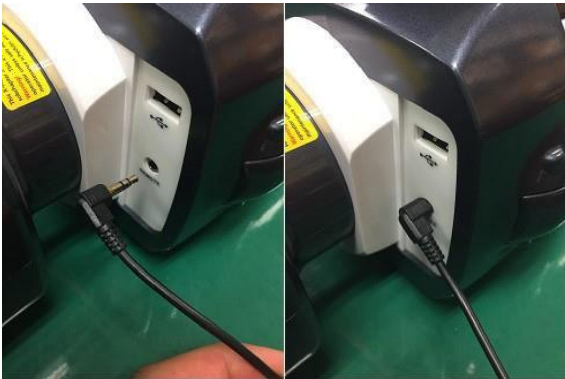
[Figure 7.14 Wired Remote Control Connection]
