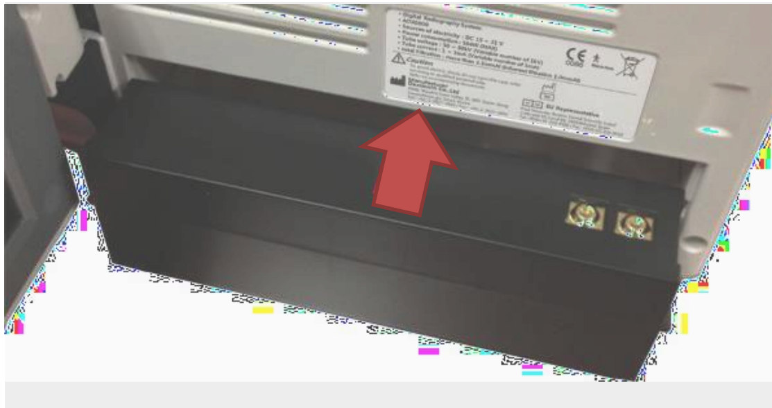
[ Figure 7.16 Inserting the Battery Pack]
