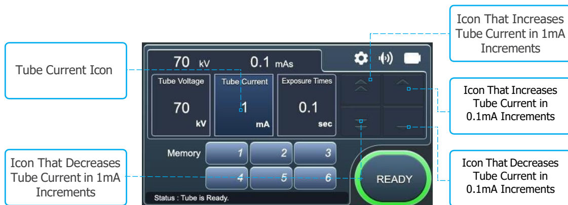
[ Figure 7.4 Icons to Change Tube Current Value]
